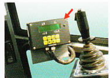
3 dimensional electric angle indicator with drilling depth and inclination
